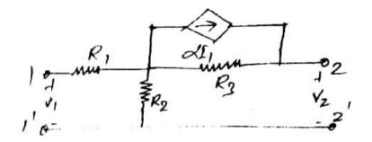
(d) For the network shown below,  $y_{11} = y_{21} = y_{22} = 2$  mho, and  $y_{12} = 1$  mho, and constant current source Ia = 1 Amp. Determine V<sub>1</sub> and V<sub>2</sub>.
