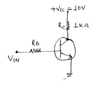
(d) If  $\beta = 100$ , determine whether silicon transister is operated in cut off, saturation or Active Region.
