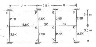
Calculate Maximum positive B.M. at the centre of span AB and maximum negative B.M. at the centre of span BC.
